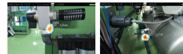
Air leaks detected from connections of pipes, valves, and other components
